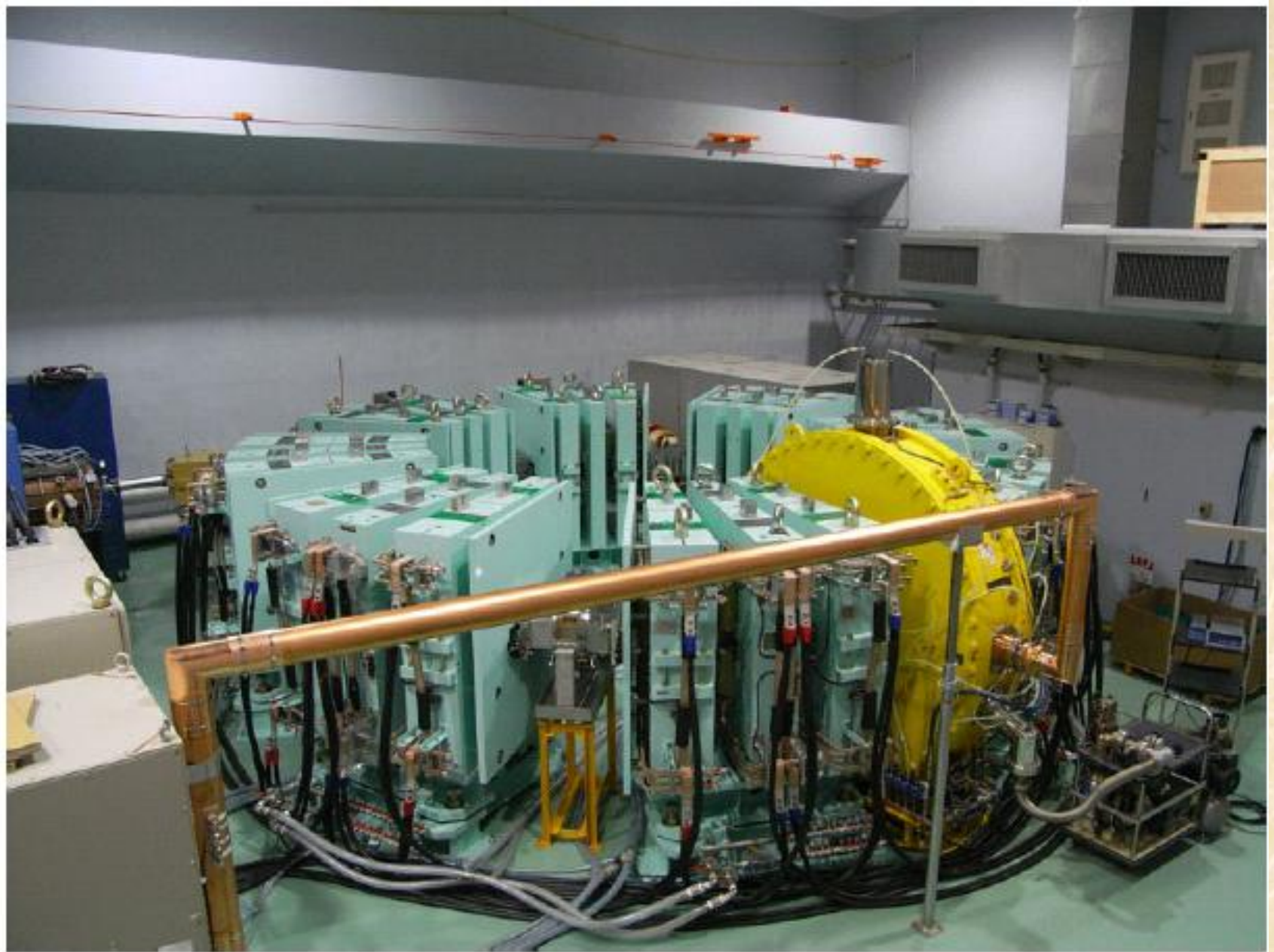
Figure 2: Photograph of FFAG-ERIT ring.
